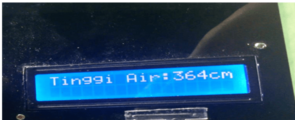
Figure 4. Real-time data output displayed on the gateway's local 16x2 LCD module
