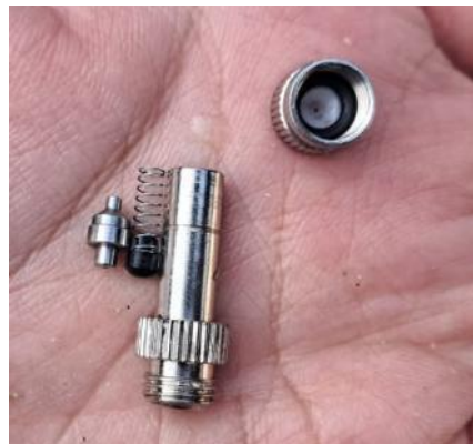
Figure 9. Misting nozzle disassembled for manual cleaning, showing the body, spring, check-valve poppet, and orifice cap.
