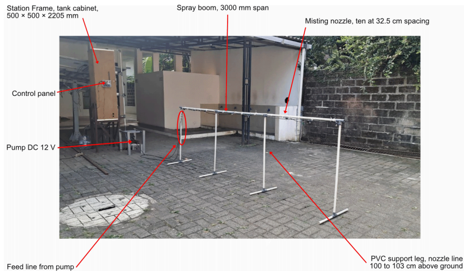
Figure 6. Assembled spray boom with labelled parts: the 3000 mm boom, the ten misting nozzles at 32.5 cm spacing, a PVC support leg, and the feed line from the pump.
