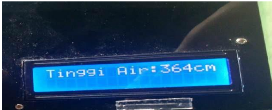
Figure 11. Display of Measurement Results Using a 16x2 LCD
